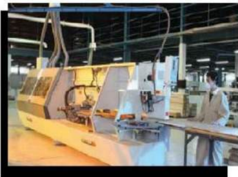
German HOLZER Edge Bander Automated CNC machine capable of panels, doors, and soft wood products
