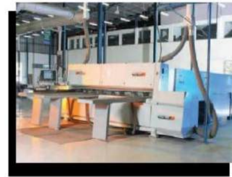
German HOLZER Panel Cutter Fully Responsible For banding edges for cutting 8 panels at a time
