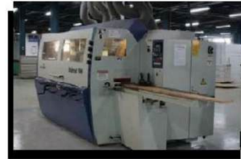
Fully automatic multipurpose spindle moulder Heavy Duty Machinery ideal for production of most joinery product's rebating, grooving, and moulding
