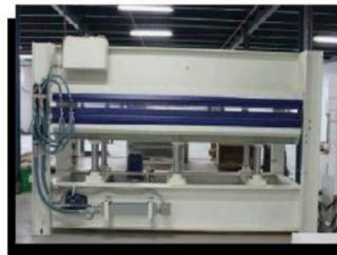
A heavy duty veneer & laminating press made with solid steel platens
