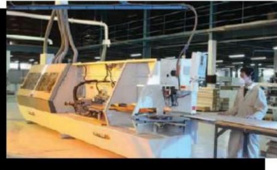
German HOLZER Edge Bander Automated CNC machine capable of panels, doors, and soft wood products
