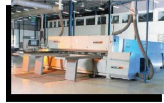
German HOLZER Panel Cutter Fully Responsible For banding edges for cutting 8 panels at a time
