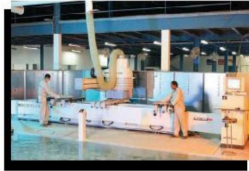
German HOLZER CNC Router Fully automated specialized in
