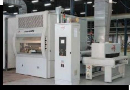
Italian CEFLA automated computerized Wood spraying 86 painting system
