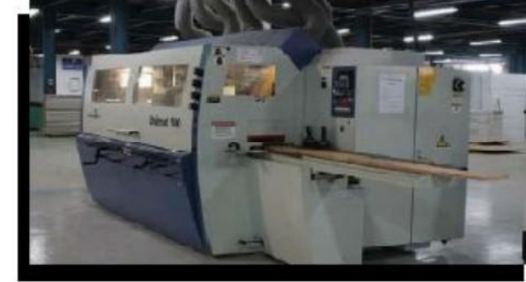
Fully automatic multipurpose spindler moulder Heavy Duty Machine ideal for production of most joinery product's rebating, grooving, and moulding
