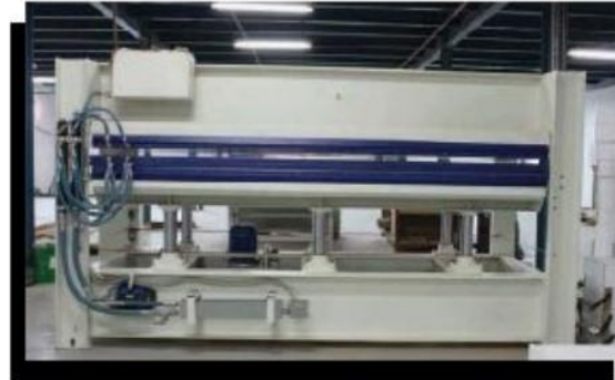
A heavy duty veneer & laminating press made with solid steel platens
